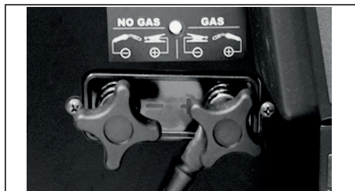
Figure 2 - Changement de tension - Unitech 328
